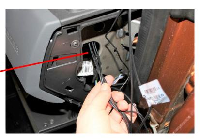
Combine the main socket, radio socket and USB socket in the box with their vehicle counterparts.
