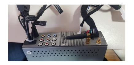
After inserting the sockets of the unit, you can install it to the vehicle with its screws.
