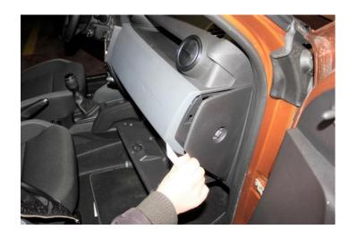
Remove the right side cover of the glove box with the help of the plastic separator.
