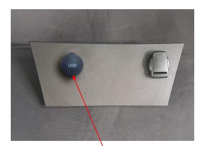
Mount the usb port on bakelite, then tighten the screw from the back.
