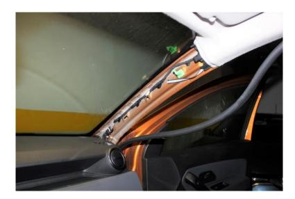
Move the microphone cable from the right gap of the glove box to the area where the unit will be installed.
