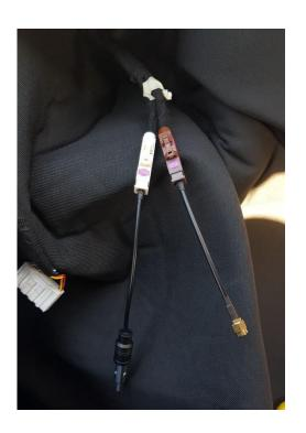
Combine the original camera connection socket, microphone socket and USB socket with their unit counterparts.
